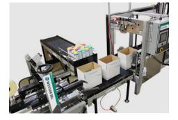
BEL 290 CASE SEALER High speed fully automatic top and bottom case sealer provides a safe and effective solution for high
