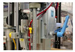
EASY MACHINE SETUP AND CASE SIZE CHANGE User-friendly pictorial guides and tool-less color coded labels and handles for convenient setup and size changes.
