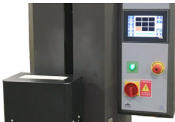
The display is full color with a high resolution touchscreen to easily change wrap counts, turntable and carriage speed and film tension. The powerful microprocessor stores recipes, user-manual and more.
