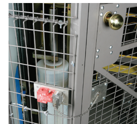
Two electrically interlocked doors on the film side allow for convenient yet secure entry to the wrapping zone.
