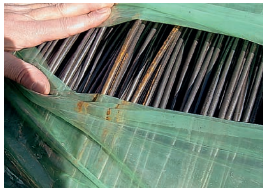
Goods after transport “without” VCI protection
