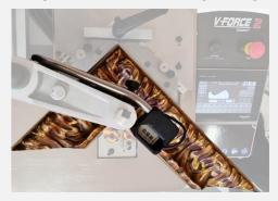
Thanks to a cutting-edge laser, you can scan your moulding and the machine will suggest you the best positions, numbers and size of wedges needed.
