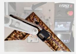
Thanks to a cutting-edge laser, you can scan your moulding and the machine will suggest you the best positions, numbers and size of wedges needed.
