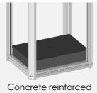
structure to absorb vibrations
